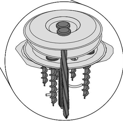
**SOPREMA FASTENERS FOR STEEL DECK APPLICATIONS**
