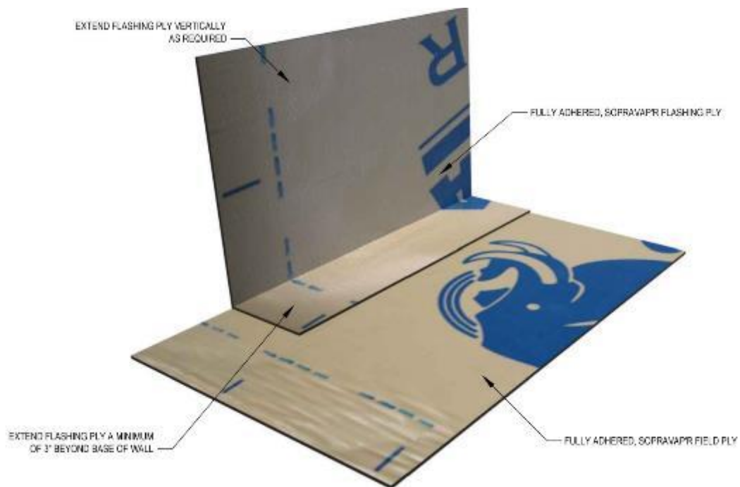
Figure 3.3.1f Fully Adhered, Self-Adhesive SOPRAVAP'R Flashing at Wall/Curb Without Cant
