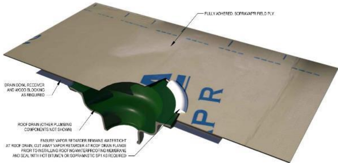
Figure 3.3.1i Fully Adhered, Self-Adhesive SOPRAVAP'R at Roof Drain
