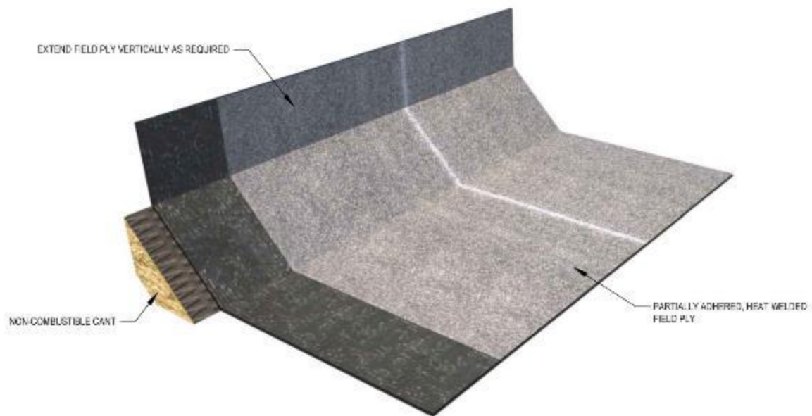
Figure 3.1.2c Partially Adhered, Heat Welded Vapor Retarder Termination at Wall/Curb With Cant
