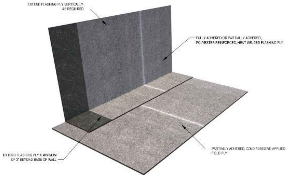
Figure 3.2.2b Partially Adhered, Cold Adhesive-Applied Vapor Retarder Field Ply at Wall/Curb Without Cant
