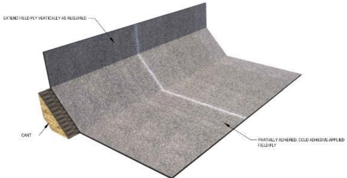
Figure 3.2.3c Partially Adhered, Cold Adhesive-Applied Vapor Retarder Termination at Wall/Curb With Cant
