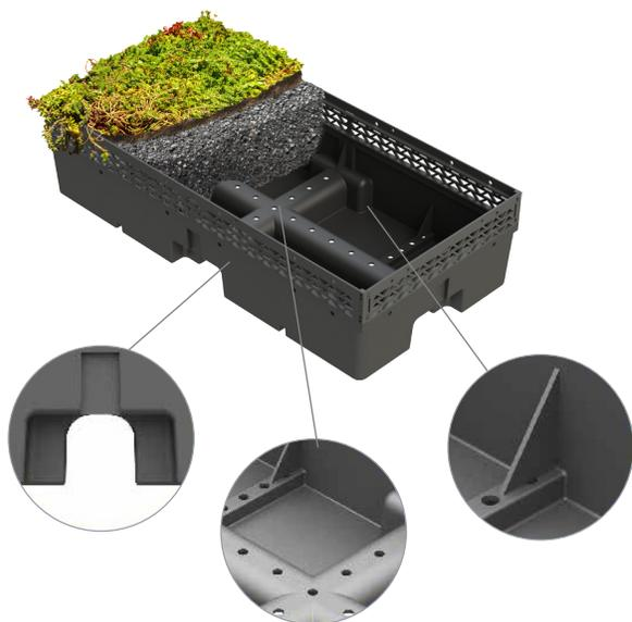
SOPRANATURE modular systems are ideal for extensive and semi-intensive vegetated roof designs. The module features built-in irrigation channels, maximizing stormwater retention. These engineered channels within the module also allow air flow throughout, mitigating wind uplift and supplying air circulation and needed oxygen to the plants' root system. In addition, these channels accommodate irrigation supply lines for all types of irrigation systems, either during or post installation.
