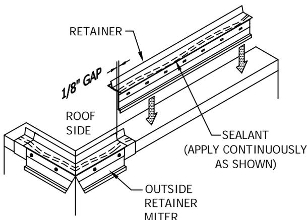
**STEP 3: Installing Retainer**
