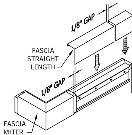
**STEP 6: Installing Fascia Straight Lengths**
