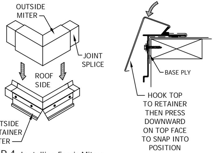
**STEP 4: Installing Fascia Miters**
