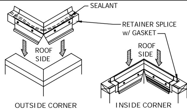
**STEP 2: Installing Retainer Miters**
