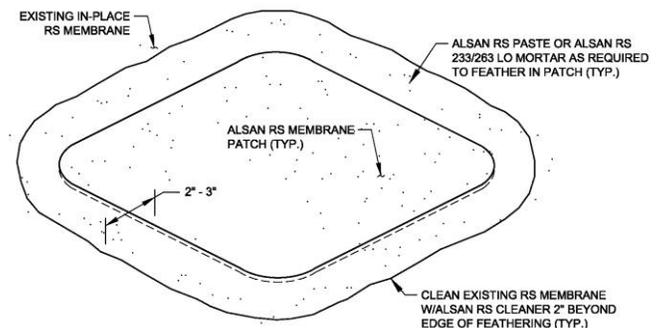
Imperfections telegraph through surfacing & finish, and therefore must be corrected before proceeding. Minor imperfections in the applied paste or mortar can be ground down before applying surfacing or finish. With a diamond cup wheel hand grinder, lightly grind the top surface of any imperfections and adjust feathering using care not to damage the in-place membrane.
