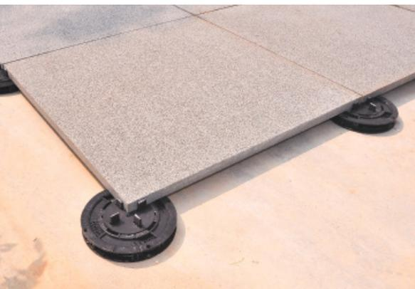
SpiraPave® pedestal is based on a unique 'step' design for supporting raised pavers and timber decking. It creates a cavity to conceal services, improves heat and sound insulation, facilitates rapid surface drainage and allows easy access to waterproofing and services. It also reduces efflorescence and algae growth and reduces paving installation costs.
