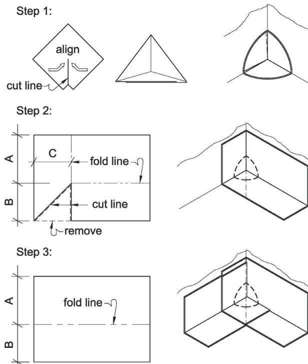
Install the pre-cut fleece corner with the overlap down using a catalyzed basecoat and topcoat of ALSAN RS resin. The "A", "B" & "C" dimensions in the diagram below represent the flashing base
