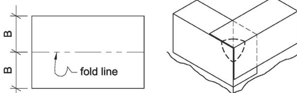
Install the pre-cut fleece corner with the overlap up using a catalyzed basecoat and topcoat of ALSAN RS resin. The "B" & "C" dimensions in the diagram below represent the flashing flange and corner wrap respectively. Once the corner is set, apply the corner flashing right and left panels as required applied in a catalyzed basecoat and topcoat of ALSAN RS resin.
