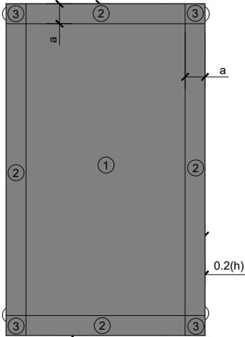
$a = 40\%$  of least horizontal dimension or 40% of eave height, whichever is smaller, but not less than either 4% of least horizontal dimension or 3ft
