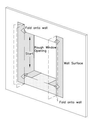
A. PRE-FOLD FLASHING INTO WINDOW OPENING WITH RELEASE LINER STILL ON.
